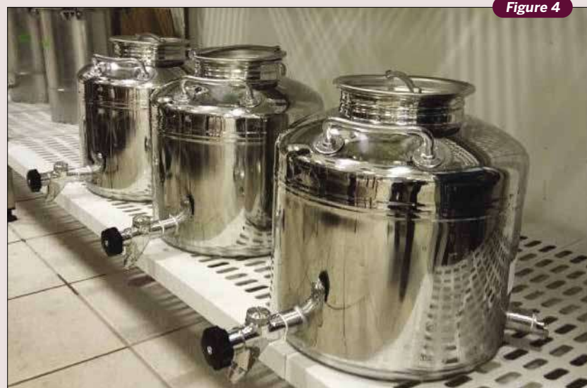
Experimental tanks equipped of three different valves, at the bottom of the tanks, all at the same level.
